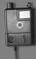
Control box and power cable
